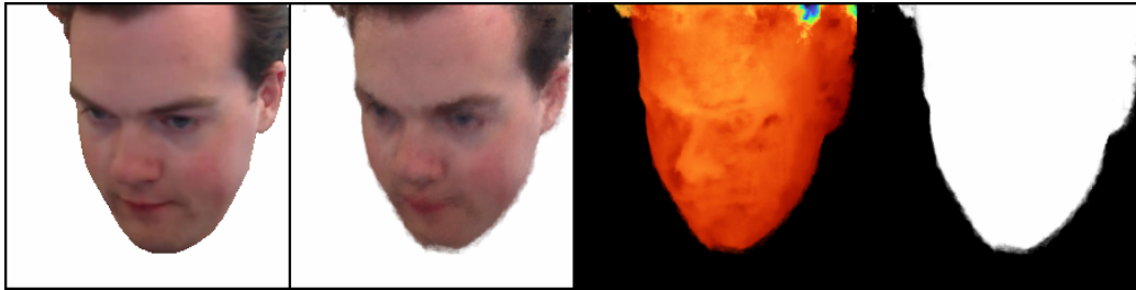
Figure 4.8: Manual alignment procedure applied to 3DMM head pose estimation result. Validation data is sharper, and the depth estimation is more consistent. From left to right: ground truth, prediction, depth estimation, mask
