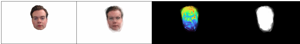
Figure 4.6: Using light-weight models for head-pose estimation is insufficient despite using additional alignment algorithms, resulting in blurred outputs. From left to right: ground truth, prediction, depth estimation, mask
