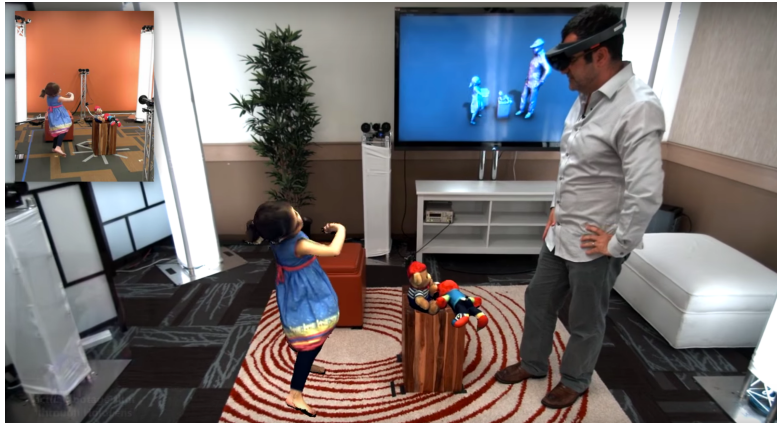
Figure 1.1: Holoportation: the augmented reality system brings two separate people into the same physical room. The system consists of eight carefully calibrated RGB-D cameras. Credits: Microsoft
